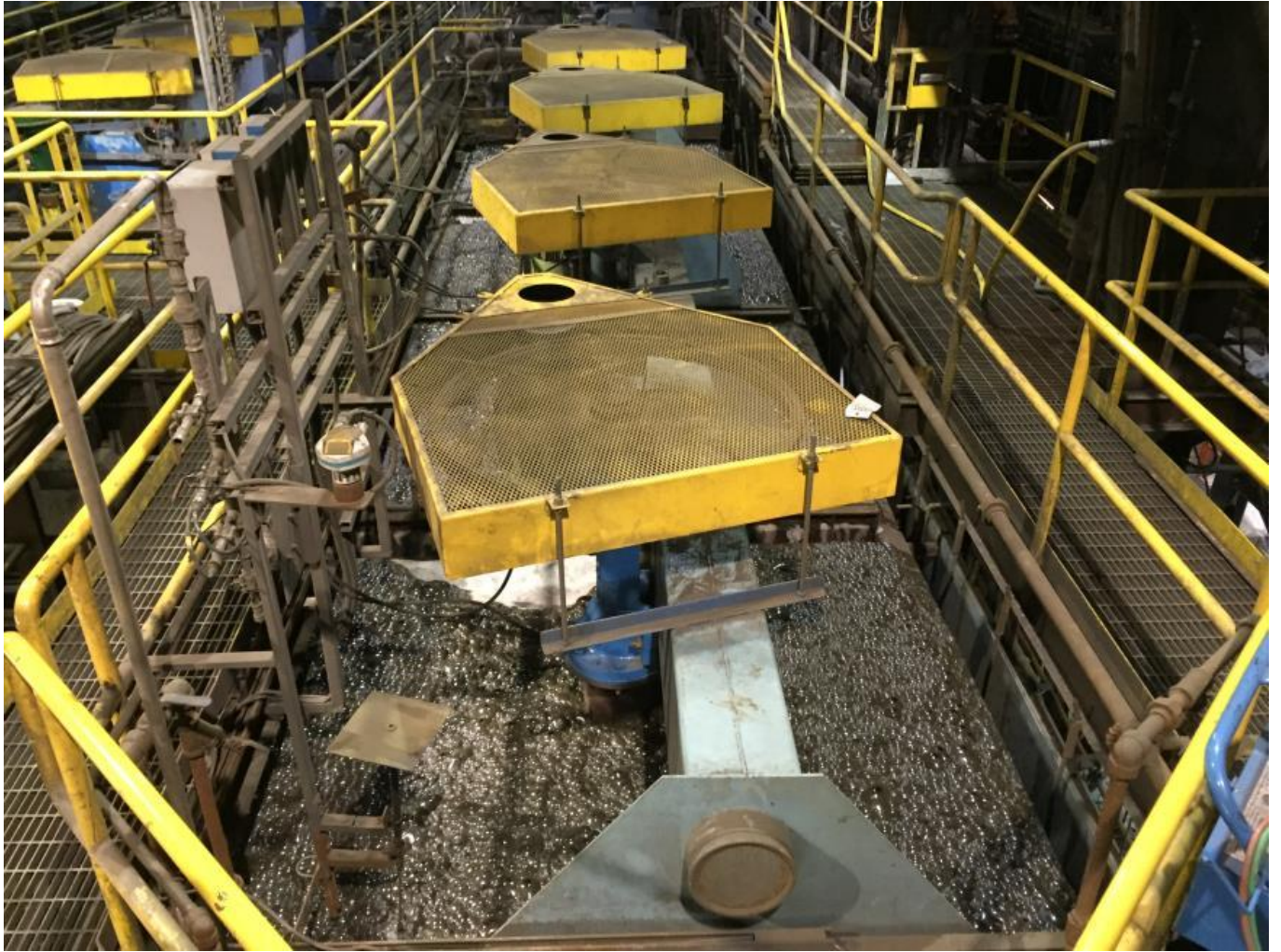
Figure 1: Caribou mill zinc flotation recovery circuit
