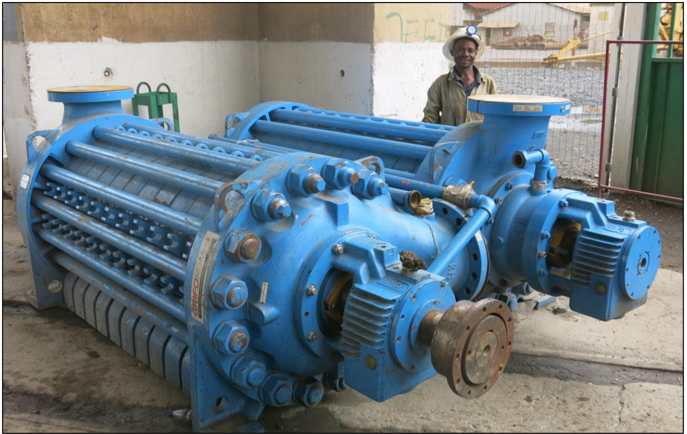
Figure 11: New Grifo centrifugal pumps to be installed at the 1,200-metre-level pump station.
