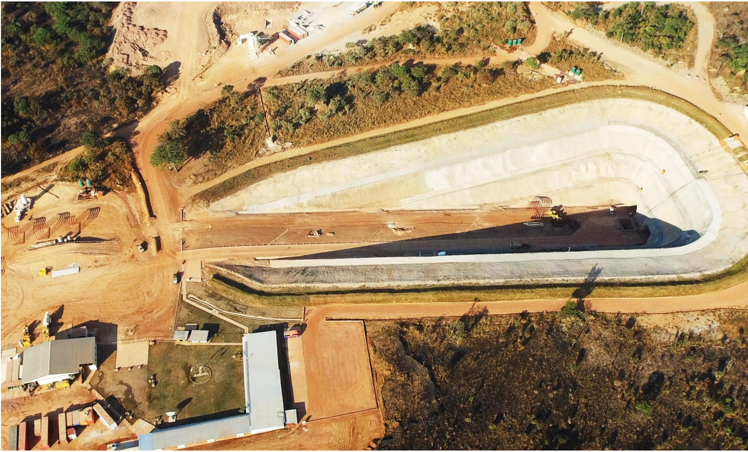
Kamoa box-cut, showing entrances to twin declines (at right) and surface facilities
