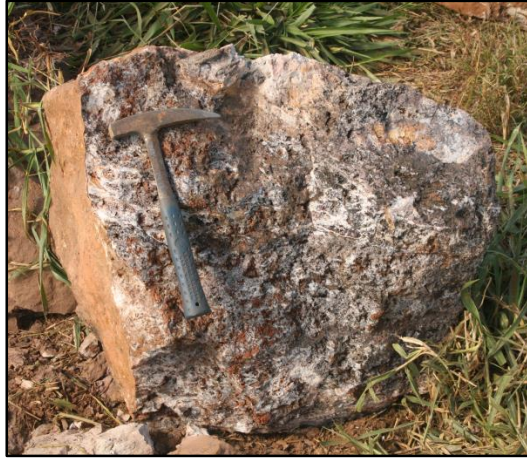
Gazetta Prospect: Variably sheared to brittle quartz veins with sulphides and boxworks (rock chip and channel sample results pending).
