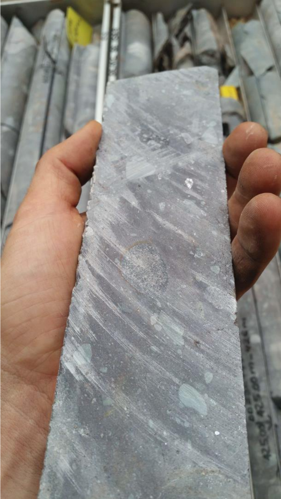
Figure 1. Drill core from DD1049 with disseminated chalcocite in diamictite at a depth of 422 metres (chalcocite is approximately 80% copper by weight).
