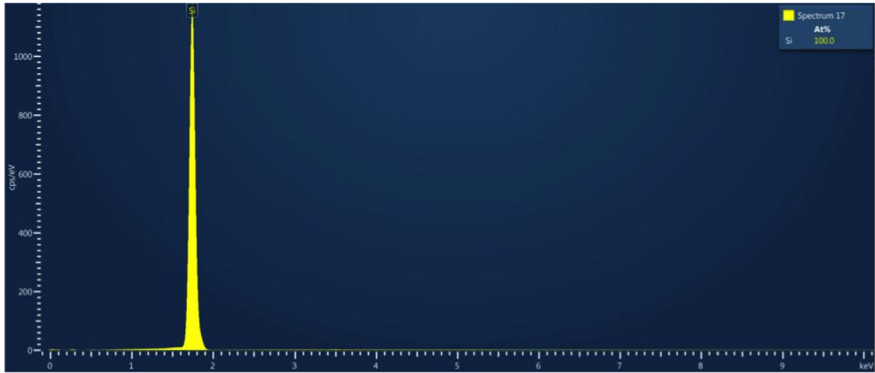
Image 2 – Example of a SEM-EDS Analysis results confirming 100% silicon 6
