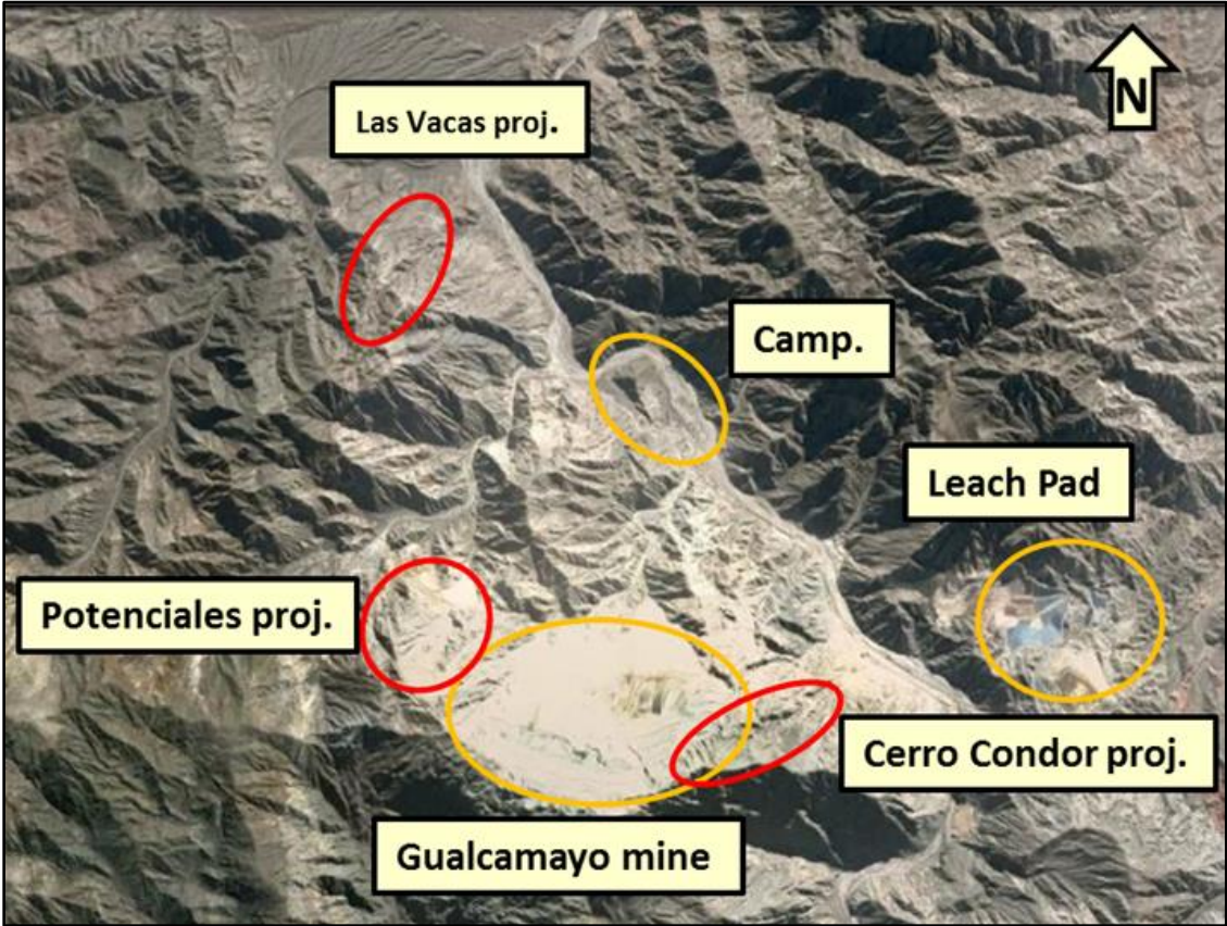
Figure 6: Plan view image of the Gualcamayo Mine open pit and close in exploration targets Las Vacas, Cerro Condor and Potenciales.
