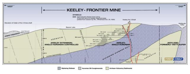
Figure 2. Reproduction of the schematic section showing interpreted geology and mine workings from archived data. Locations and scale are approximate.
