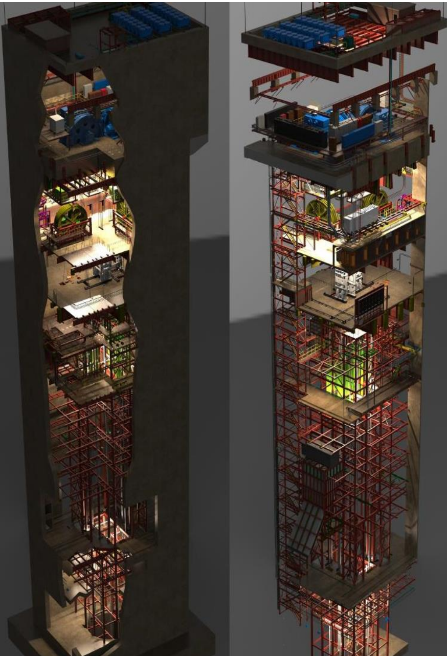
Figure 3: Illustration shows two perspectives of Shaft 2's 103-metre-tall concrete headgear, the hitch (foundation) and internal permanent hoisting facilities.
