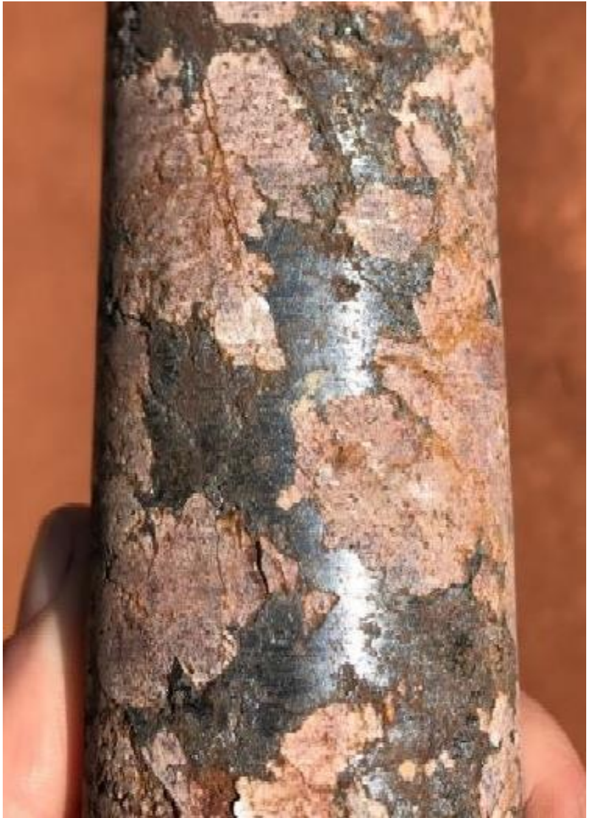
Figure 10: Massive chalcocite in a recent drill hole from Kakula West. Chalcocite is approximately 80% copper by weight.
