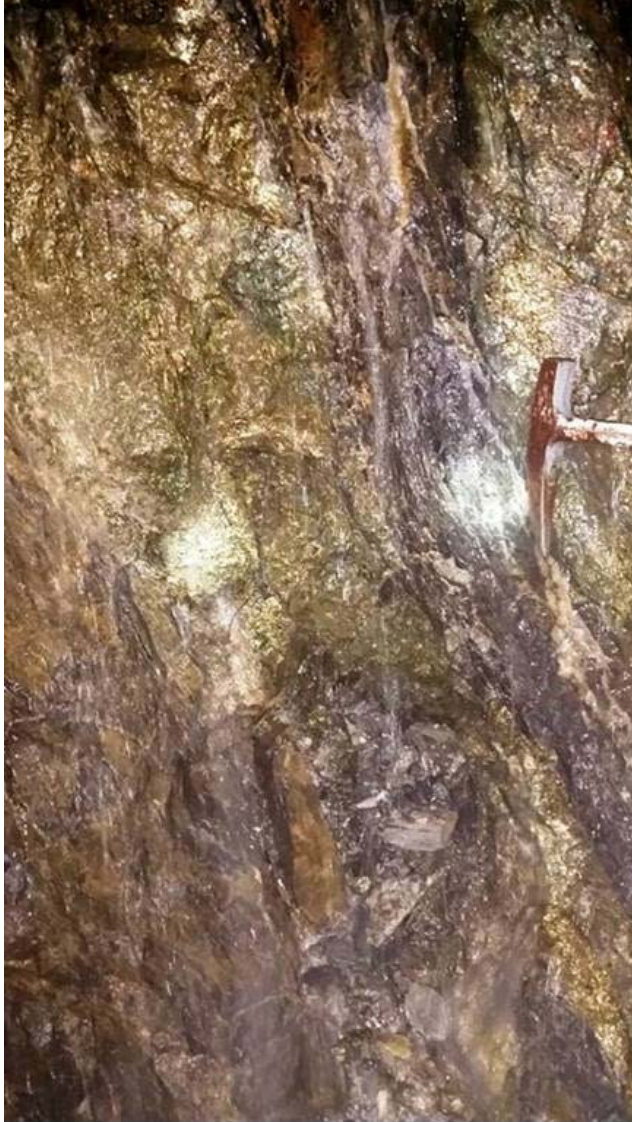
Photograph: Massive chalcopyrite present in the face of a drive on the Kora Lode currently being mined at the Kainantu Mine. This entire face averaged 4.1 metres @ 8.86 g/t Au, 20.9 g/t Ag and 1.14% Cu.
