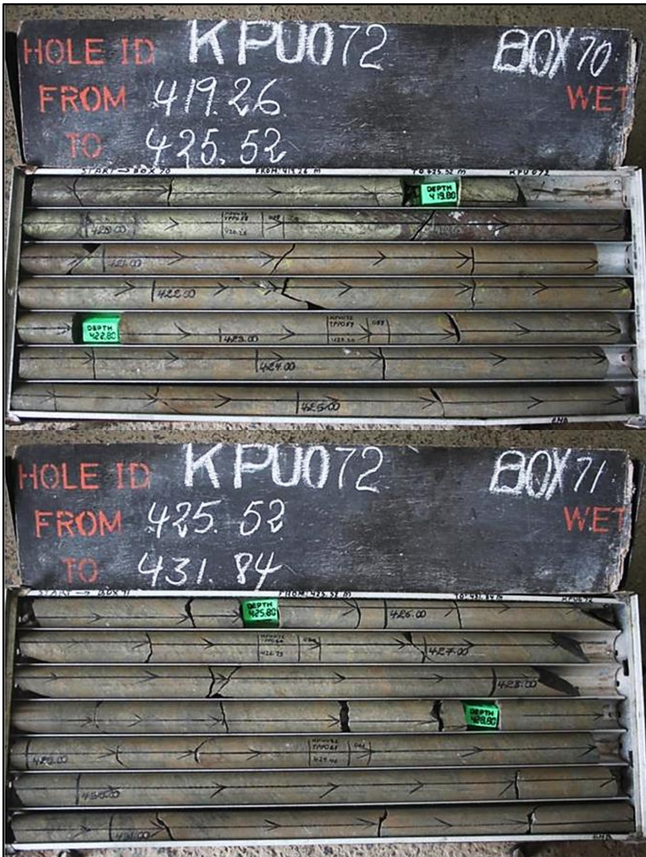
Figure 6: Discovery hole KPU072 with mixed chalcopyrite and sphalerite to 420.55 metres and massive sphalerite from 420.55 to 431.84 metres.
