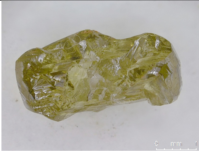
A) Sample J1-1: Greenish-yellow transparent broken complex crystal, size fraction -2.36 \text{ mm} +1.70 \text{ mm} , 0.1385 carats
