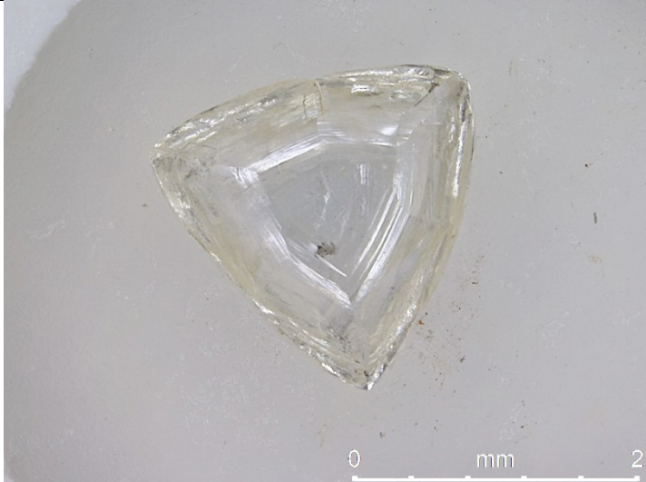
C) Sample J3-1: White transparent octahedron, size fraction -2.36 \text{ mm} +1.70 \text{ mm} , 0.0707 carats
