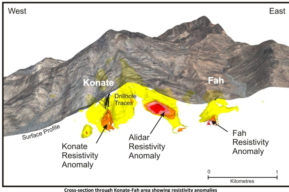
Cross-section through Konate-Fah area showing resistivity anomalies
