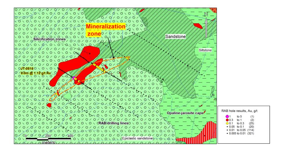
Figure 4 – Zhanatobe 2010 RAB Drilling Results: the newly discovered mineralization zone in the Northern area
