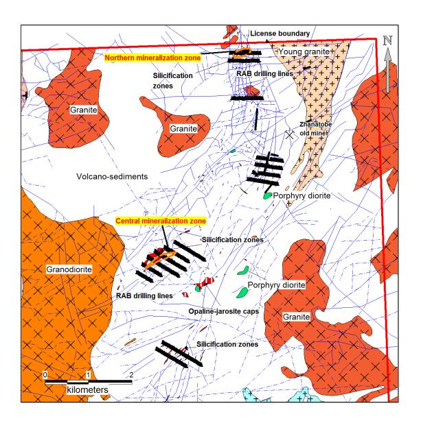
Figure 3 – Zhanatobe 2010 RAB Drilling Results: the newly discovered mineralization zone in the Central area
