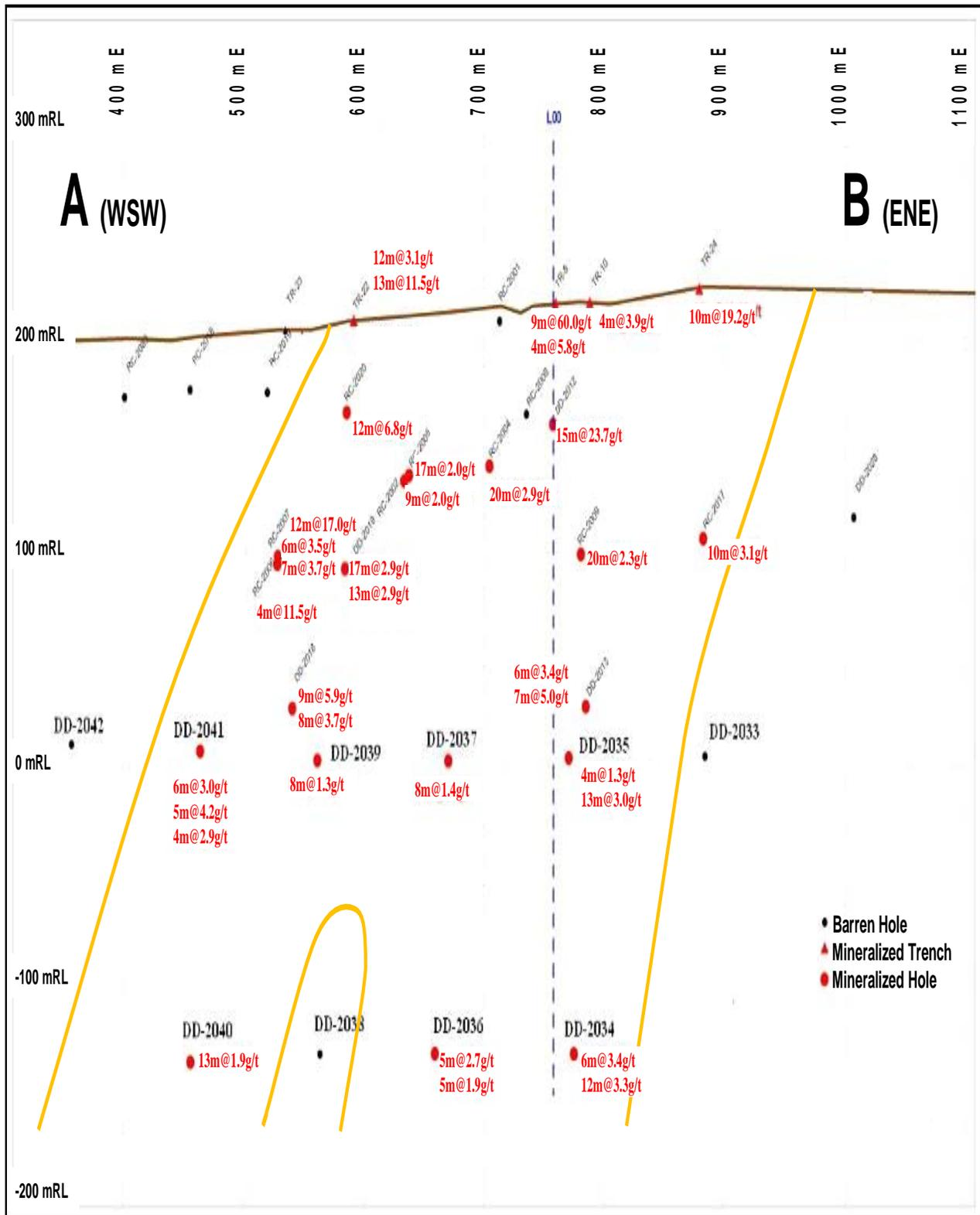
Figure 7 – Schematic long section of Boto 5 highlighting potential SW-plunge of mineralisation. Note that the mineralized zone dips 80° to the north and that the section is oblique to the drill grid above 0mRL.
