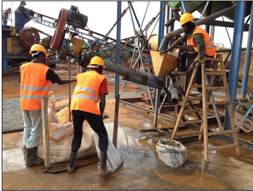
Photo5: Pre-production: Spiral concentrate product, coming out of screw concentrator.
