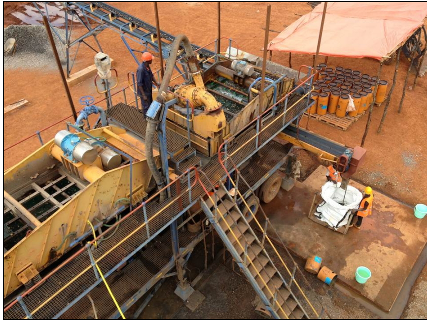
Photo 3: Pre-Production: DMS module-malachite concentrates to the right into the bag, low-grade gravel to the left.
