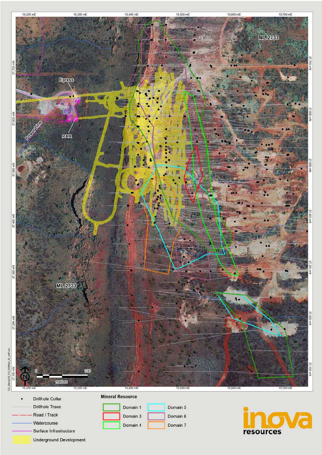
Figure 3: Plan showing location of drilling, outline of Mineral Resource domains and infrastructure
