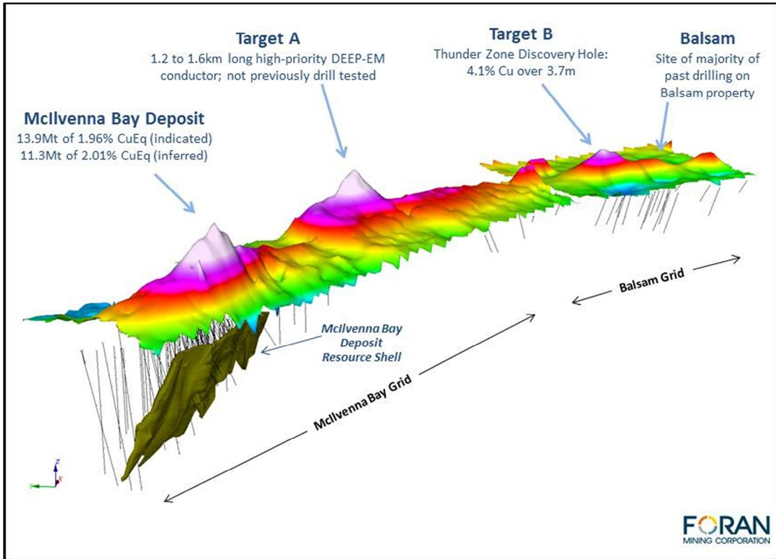
**Figure 2.** DEEP-EM conductor response relief map for McIlvenna Bay and Balsam Grids, looking east. Data is gridded mid- to late-time EM channel 20 - component X utilizing a compressed linear colour scale; drill hole traces shown in black.
