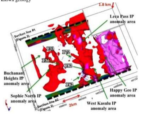
Figure 2: The 2013 IP survey penetrated to greater depth covering a number of untested areas All historic holes highlighted have not penetrated to the target depth of IP targets but have returned copper and/or copper-gold anomalies/mineralization
