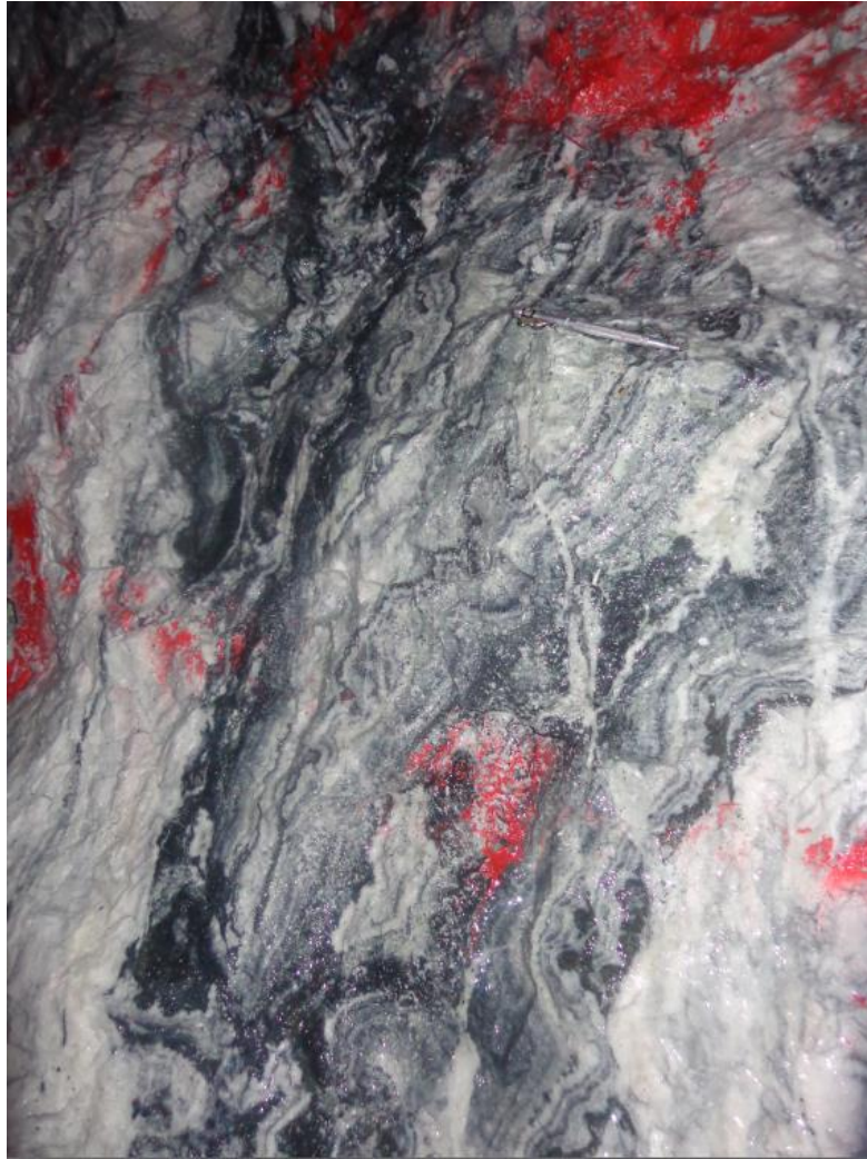
SD-2285SE – CHIN_012: Inca Vein (Detail) – Breccia-Cockade-Banded Texture - Sample UN-P097: 0.80m at 78.89g/t gold and 7,695g/t Silver or 207.13 g/t Au_Eq
