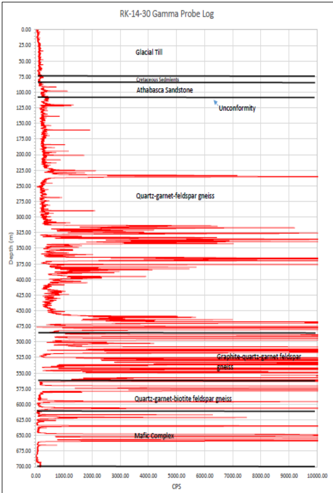
Fig 2 Arrow, RK-14-30 (gravity target), 2PGA-1000 downhole probe results (capped)
