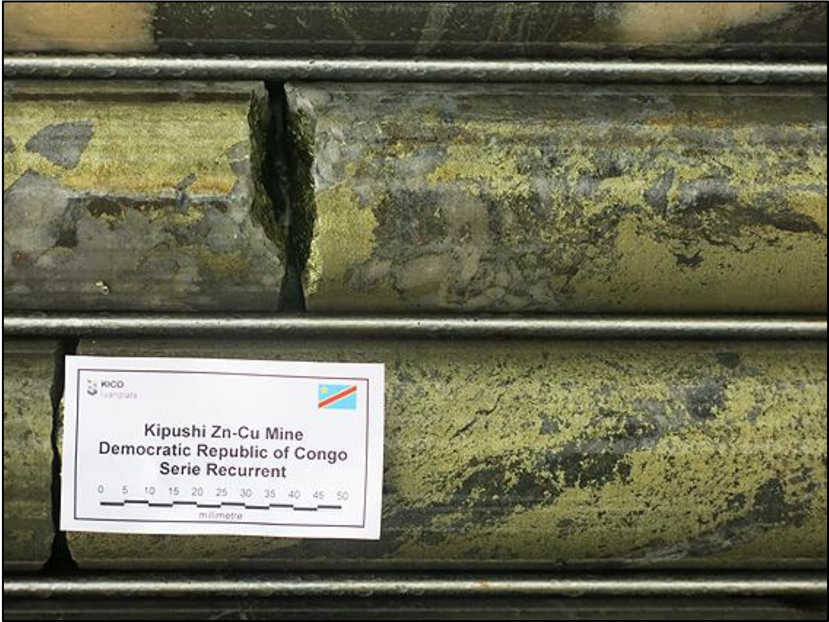
Figure 8: Core sample of chalcopyrite intercept from 59.7 to 62.0 metres in Hole KPU004.
