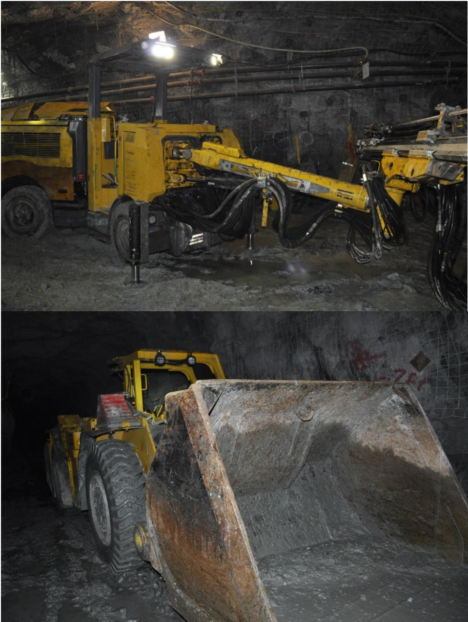
Figure 3: Newly Acquired Jumbo Drill and Scoop Tram on the 183-Metre Level
