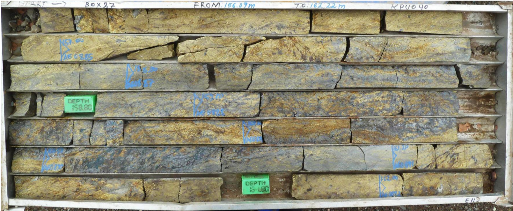
Figure 6: Close-up photographs of massive copper sulphides (chalcopyrite and bornite) with high silver and gold values in drill hole KPU040 through the Big Zinc zone.
