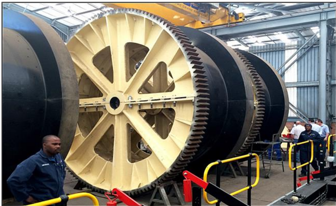
Photo 4: Stage-winding drums to be used in the sinking of Shaft #1.
