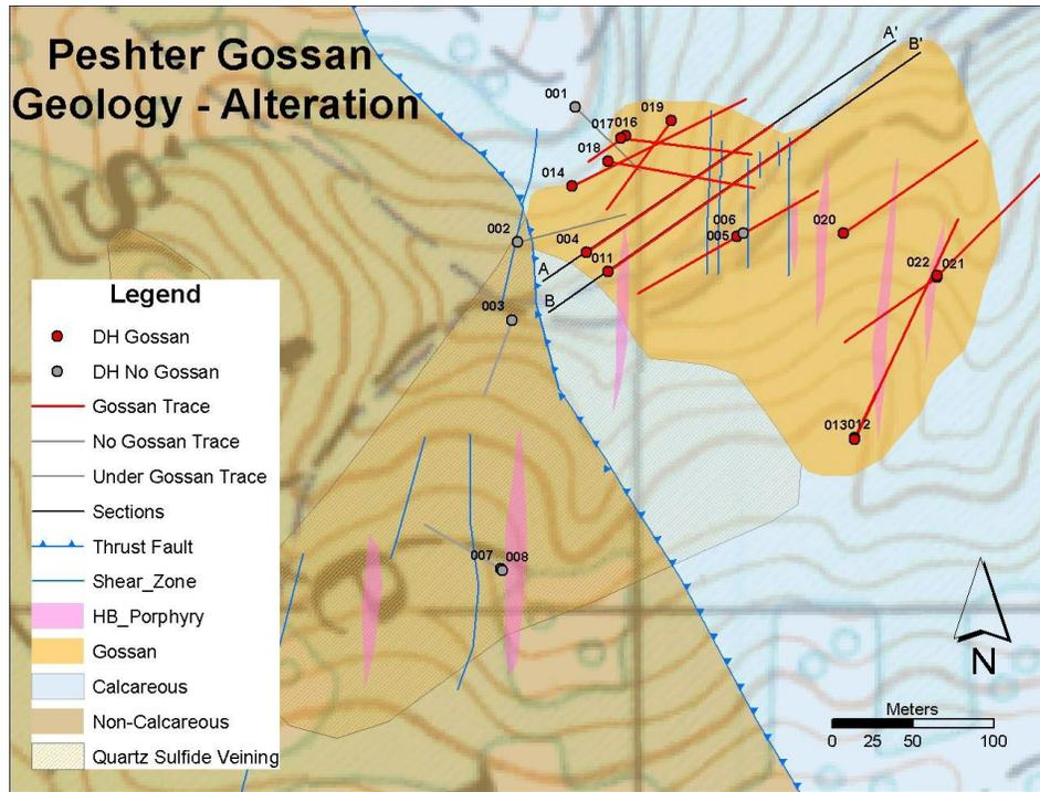
**Figure 1.** Plan view map of drilling in the Peshter Gossan Zone. Note the locations of SLV014, SLV004, and SLV011.
