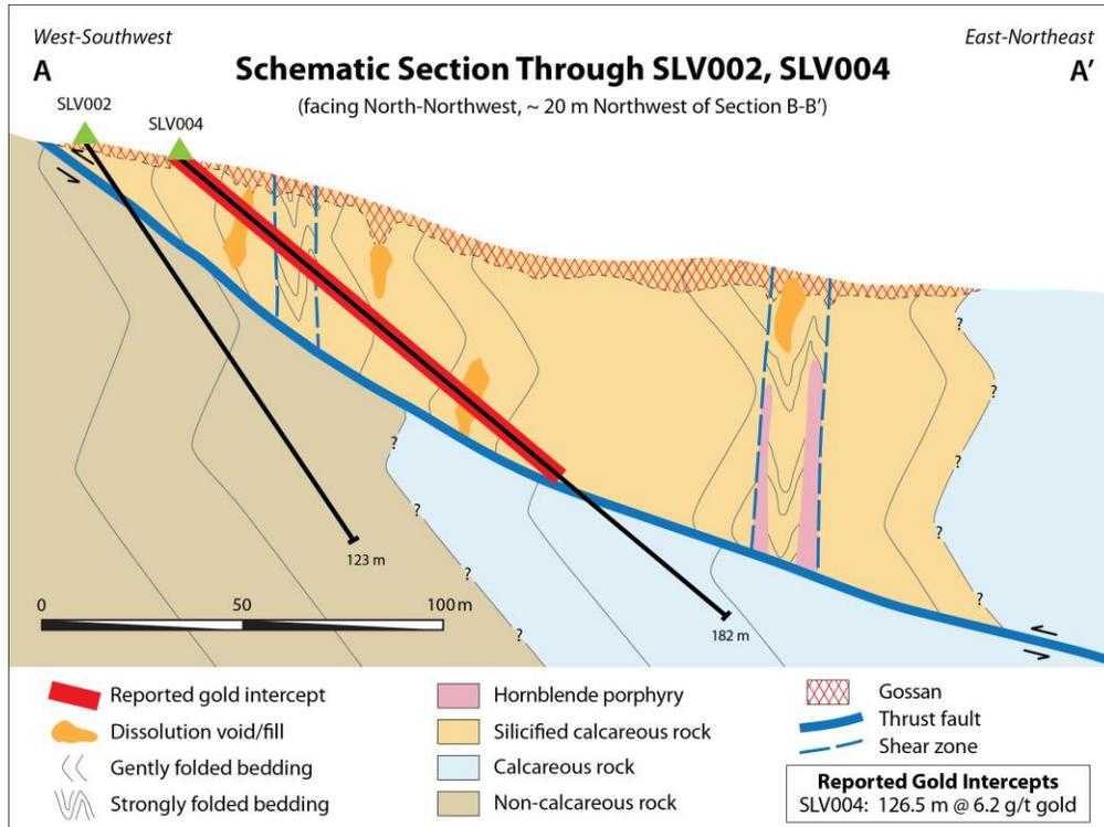
**Figure 2.** Section through SLV002 and SLV004, showing previously reported gold intercept.
