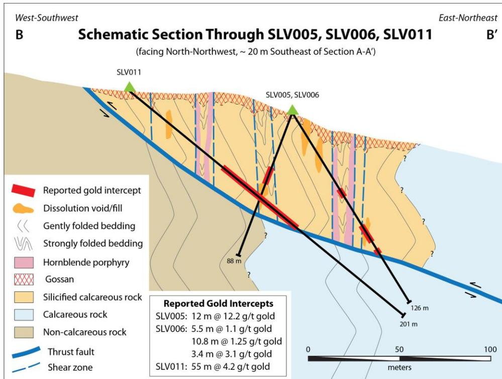
**Figure 3.** Section through SLV005, SLV006, and SLV011 showing previously reported gold intercepts. SLV005 and SLV006 lie approximately 20 meters in front of this section, and are shown for interpretative purposes.
