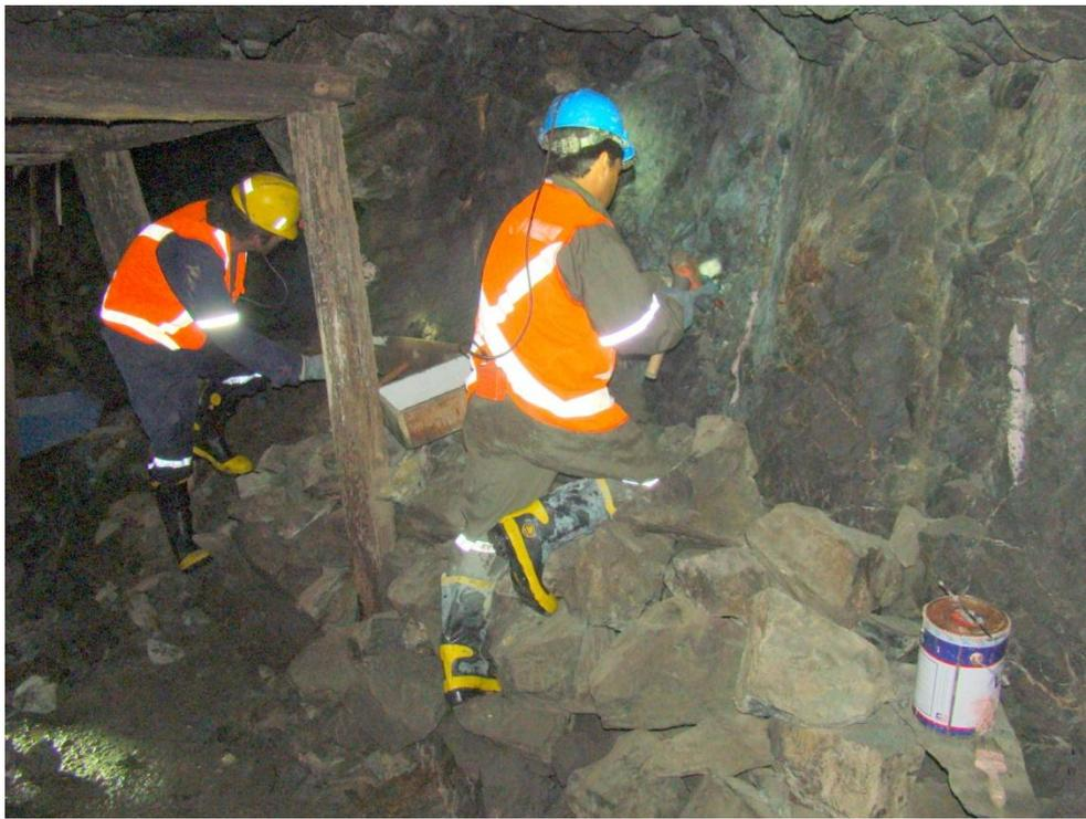
STOCKWORK AND VEINLET COPPER SULPHIDE MINERALIZATION IN OLD MINE WORKINGS AT LA HIGUERA BEING CHANNEL SAMPLED
