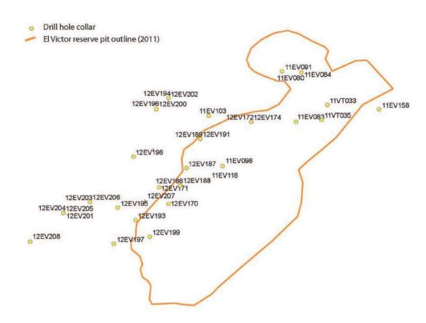
Figure 1: Previously unreleased El Victor North drill hole locations
