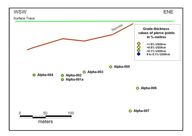
A provisional long section of the Aricheng Alpha structure shows the distribution of grade-thickness values (the product of the width of the mineralized interval and its  $U_3O_8$  grade in %) on a vertical projection of the structure. The coloured diamonds demarcate the pierce points on the structure. A pierce point is the approximate location at which each bore hole intersects the structure.
