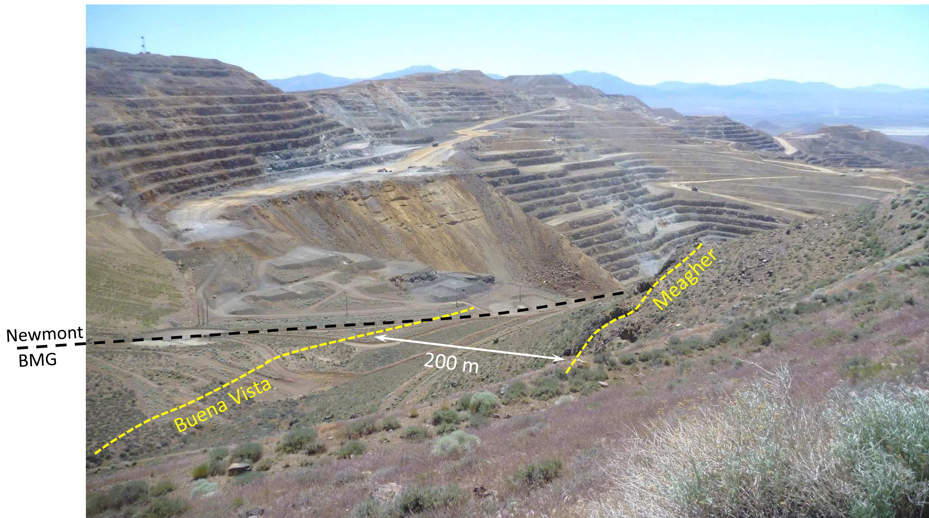
Buena Vista – Meagher Zone, southwestern portion of the Lewis Property, showing north-trending and west-dipping fault zones. These high-grade Au-Ag structures (yellow dashed lines) extend to the south across the claim boundary (black dashed line, Newmont / BMG) into the Fortitude open-pit. Maximum rock-chip assay values for these areas include 24.7 g/t Au and 359 g/t Ag for the Buena Vista and 12.3 g/t Au and 5600 g/t Ag for the Meagher. The same favorable rock units that host the Fortitude deposit lie about 100 to 250 m below surface in the Lewis claim area. Photograph taken looking south-southeast.
