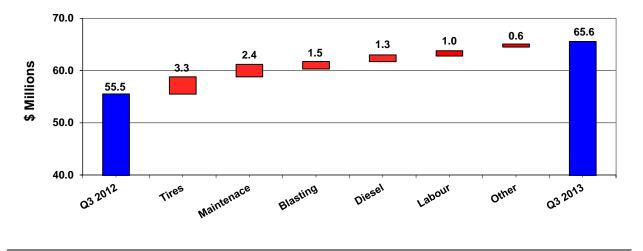
The increased cost of mining activities is primarily related to the increased tonnage moved as the higher density material incurred higher diesel and blasting costs. Other increases include higher tire requirements of the expanded CAT 789 fleet and increased maintenance of the Hitachi shovel, CAT 789 and DR460 drill fleets introduced in 2011 and 2012. Labour costs also increased as a result of wage increases provided for in the new collective bargaining agreement ratified in December 2012.
