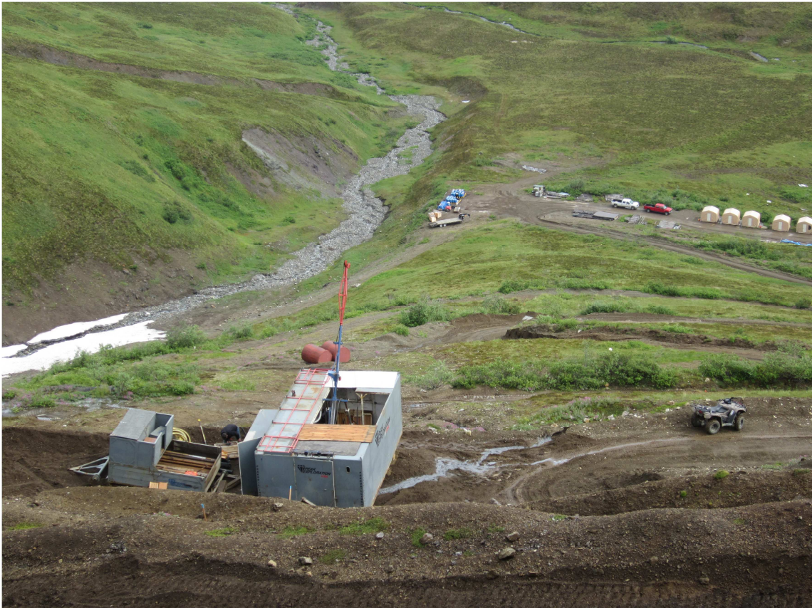
Drilling diamond core hole CD15-01 at the Caribou Dome Copper Project, July 2015.
