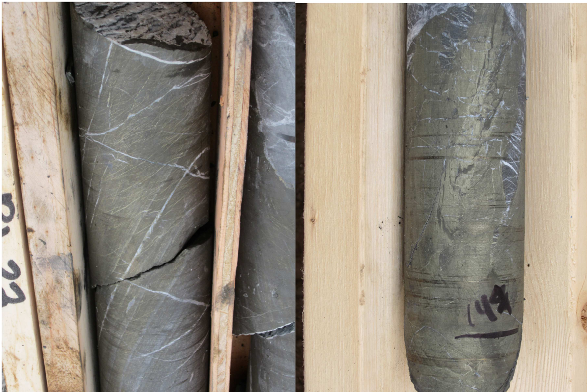
RHS: Heavily mineralised sediments intersected at 44.5m depth in CD15-01; LHS: Semi-massive sulphides intersected at 44.8m depth in CD15-01. (HQ-sized diamond drill core; 63.5mm diameter)
