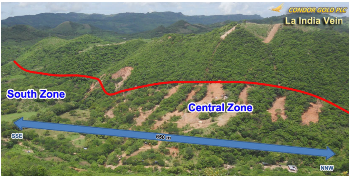
View of the surface expression of the old mine workings on the Central Zone of the India Vein with trenches and drill collar locations shown.
