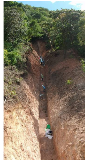
Trench sampling on the America Vein to test for gold mineralisation in the wallrock of the historic mine workings.
