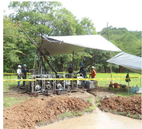
Diamond core drilling on the La India Project.
