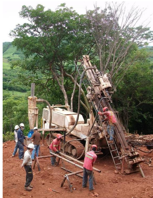
Reverse Circulation drilling on the La India-California trend.
