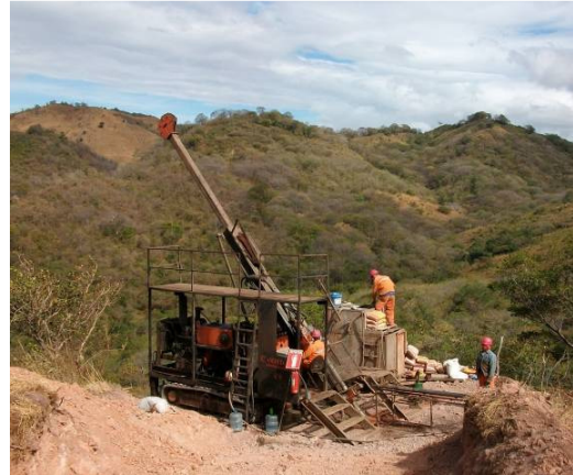
Diamond core drilling on the La India-California trend.
