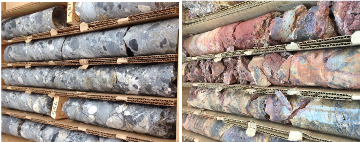
Figure 2. Core from the upper Tertiary hosted mineralization on the left and the lower Paleozoic limestone/sediment hosted mineralization on the right - Main Zone, Mother Lode Deposit.
