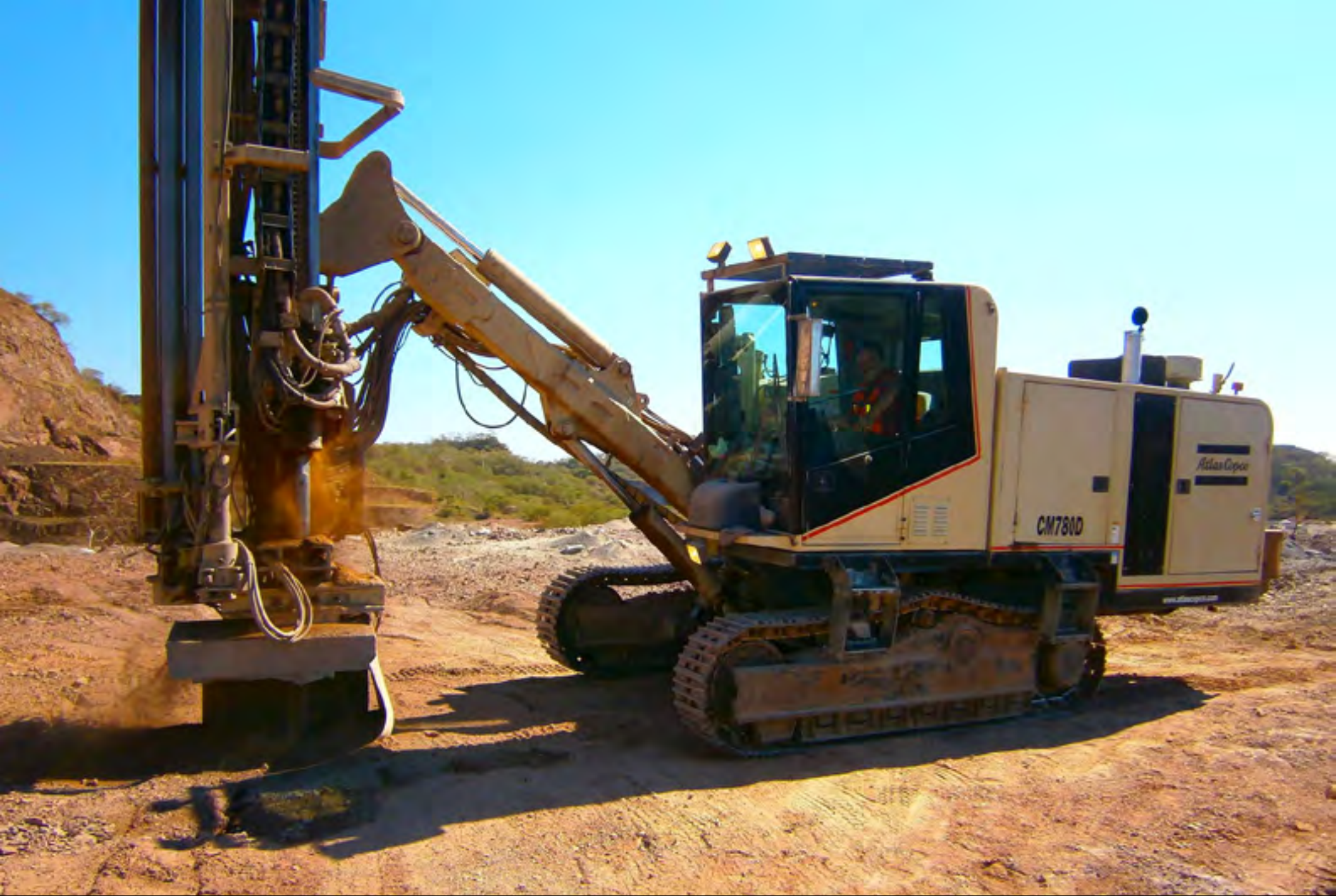
Blast hole drilling within the open pit.
