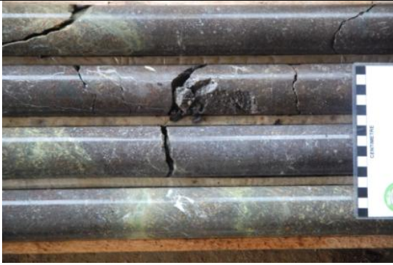
Hole RZDDH10-07: Misahualli feldspar porphyritic andesite, haematite pervasive then epidote-carbonate alteration overprint @646.5m
