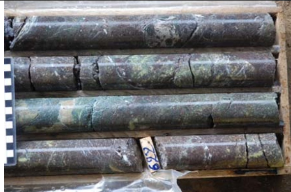
Hole RZDDH10-07: Faulted/sheared Misahualli, ep-chl alteration after ht @ 622m
