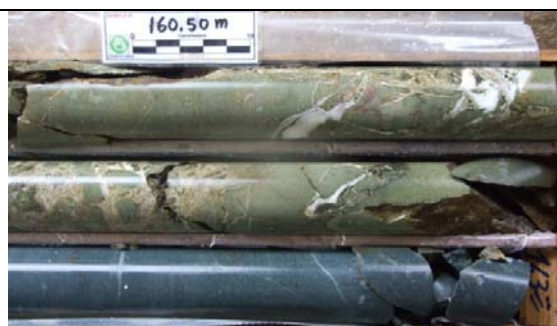
Hole RZDDH10-07: Magnetite destructive epidote-chlorite alteration with zoned quartz-carbonate-sulphide veins in Fruta andesite
