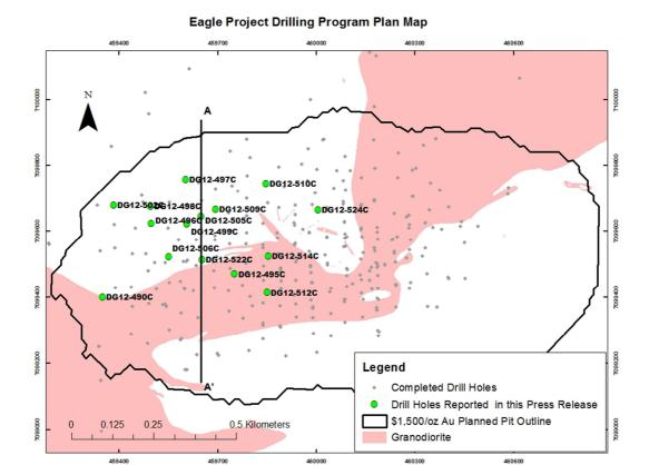
Holes angle approximately -60 degrees to the north and south to cross-cut the steeply dipping quartz-gold vein sets
