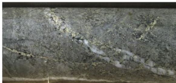
Alteration and different generation of chalcopyrite veins in F98A (628m)
