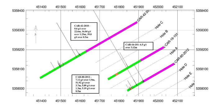
Figure 1: Diamond Drill Plan in vicinity of Hole CAR-16-101. Lettered holes are planned and not drilled.
