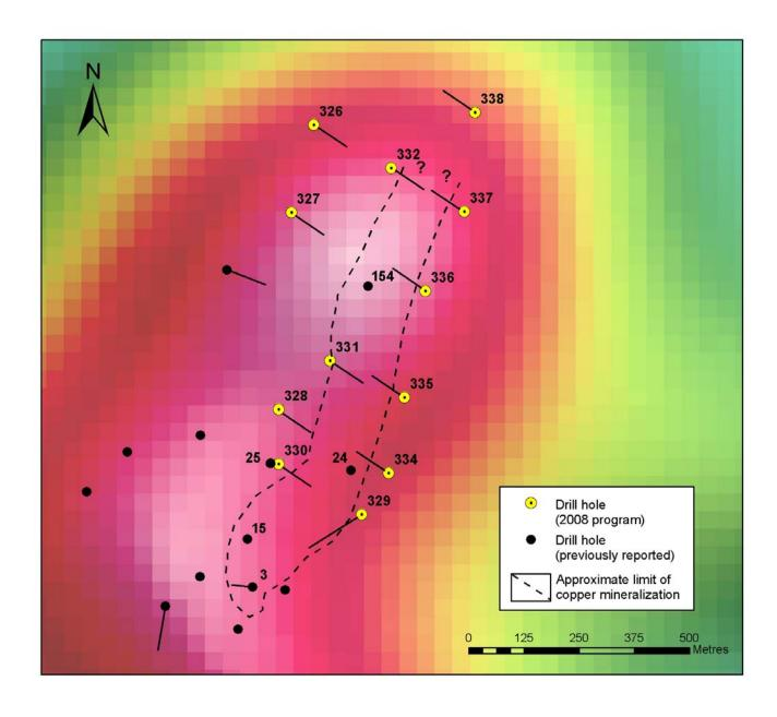
**Figure 1**: FALCON<sup>TEM</sup> gravity image showing the Iris Norte zone. The mineralized zone is 100-200m wide with a strike length of approximately 1000m. The drill holes are widely spaced and the mineralized zone remains open to the north.
