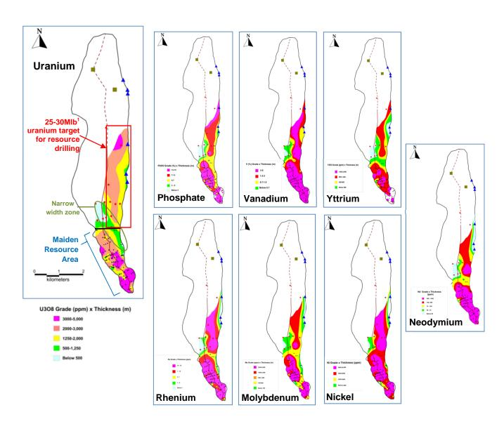
Figures show the canoe-shaped fold at Berlin flattened out. Coloured dots show the points at which bore holes intersected the mineralized layer. Grade-thickness values have been coloured to show the general distribution of the different commodities along the Berlin trend.
