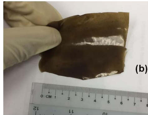
Figure 1 (a) shows the penetration processes of different ionic compounds through the GPURE GPM membrane, and (b) shows the GPURE GPM 6cm x 6cm membrane.
