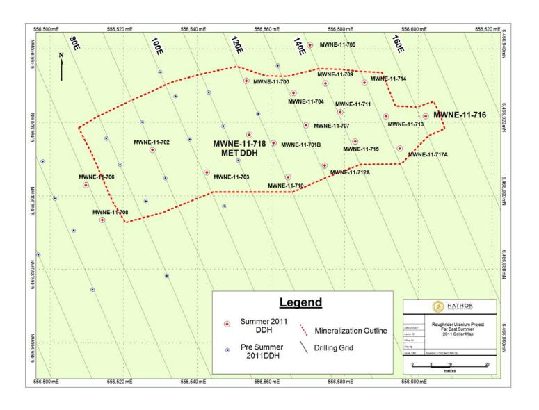
Figure 1: Grid line plan map of Far East Zone at Roughrider Uranium Deposit, with drill holes completed during 2011 winter (unlabelled) and summer (labelled) drill programs. Simplified from Figure 3 in Company's news release dated September 20, 2011.
