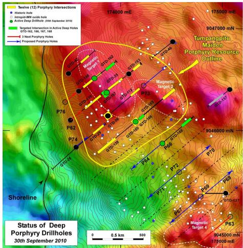
**Drill status plan:** Collars of oxide holes shown in white and blue. Deep drill traces shown in black, and proposed in blue. Those holes that have been completed are shown in yellow bars, and those in progress shown in green bars. The main porphyry copper-gold zone is outlined in the yellow solid line. Background image is reduced to pole heli-magnetics.
