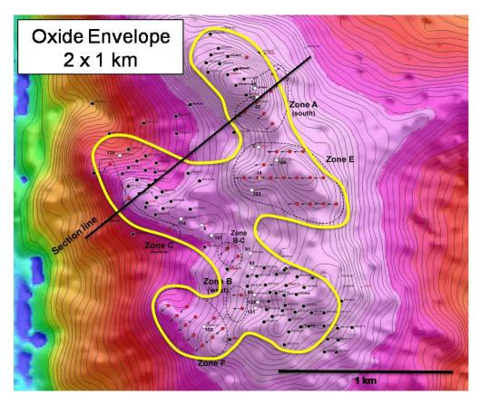
The diagram above illustrates the drill holes (marked in black) that define the existing resource estimate. Red drill holes are completed, and are expected to add further ounces in an additional 2010 estimate which will form the basis of the PEA. Significantly, results from newly drilled zones E and F will be added. The yellow outline defines the currently identified near-surface oxide and transition mineralised area.
