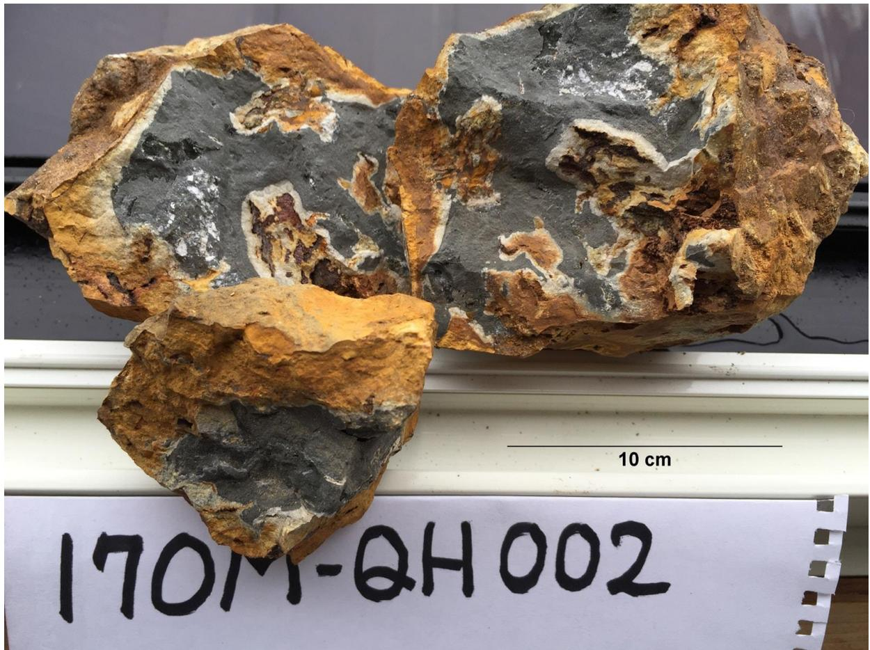
*(Figure 3: Sulfide-bearing siliceous sinter material taken from the base of the Omu sinter terrace, a fossil hot spring deposit. The high precious metal content of this sample bodes well for potential in the structural feeder beneath the terrace.)*
