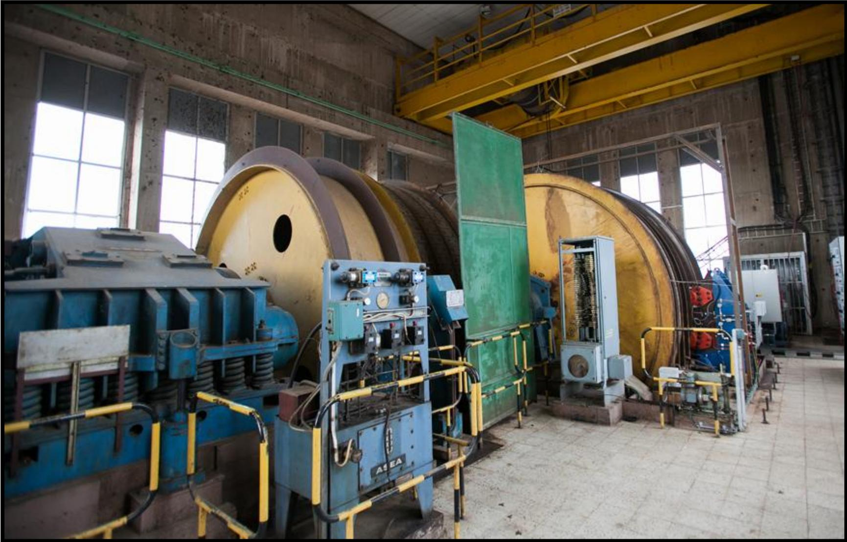
Figure 5: Newly installed winder control centre at Shaft 5.
