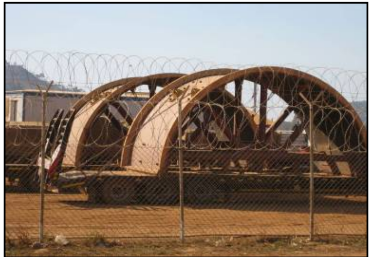
SAG Mill Shell on Site
