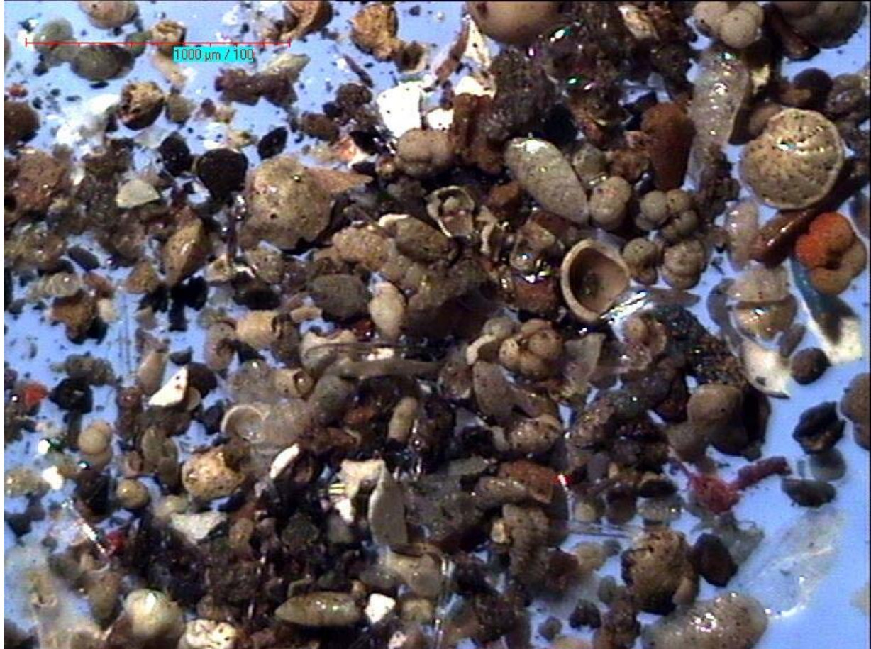
Microscopic pictures of Tailings (binocular 100 x magnification)
